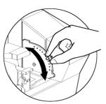
Open Cover, and adjust lever to correct position. Repeat for different card thickness. (Factory setting is for 30mil (0.762mm) card thickness). See diagram below:
